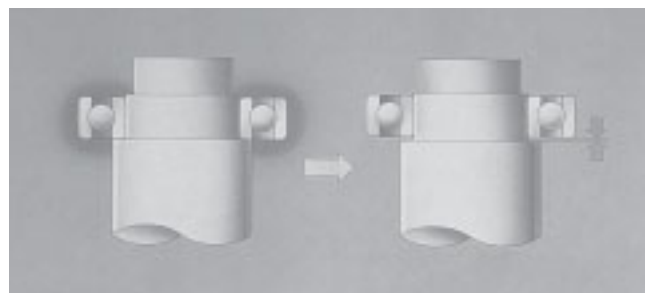
● Figure 9.3 Shaft Shoulder Gap After Cooling
